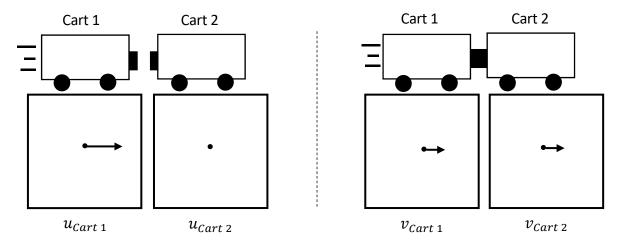
The vector diagrams above illustrate that before the collision Cart 1 had an initial velocity,  $u_{Cart\ 1}$ , and collided with Cart 2, which was at rest, and that after the collision Cart 1 had a final velocity,  $v_{Cart\ 1}$ , and Cart 2 had a final velocity,  $v_{Cart\ 2}$ .
