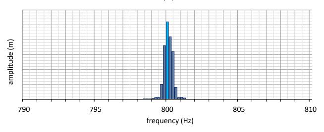
The student then attached the speaker to a string and rotated it in a circle at a constant speed while it was still set to give a frequency of 800 Hz. The circular path was horizontal and pointed directly towards and away from the microphone as shown in the diagram. The sound was recorded as before.
