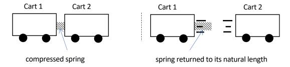
The compressed spring has a spring constant of  $11 \text{ N m}^{-1}$  and is compressed by 3 cm. The total mass of cart 1 and the spring is recorded as 330 g and the mass of cart 2 is recorded as 295 g.
