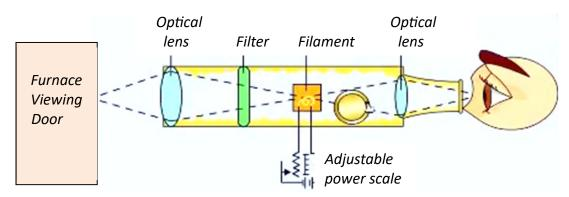
There are three possible results with the optical pyrometer: filament too bright, filament not bright enough and filament matching the furnace colour. When the filament seems to disappear the temperature of the filament matches that of the furnace and a reading can then be established.
