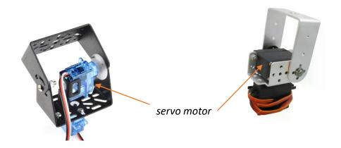
Mechanism to rotate the camera unit:
