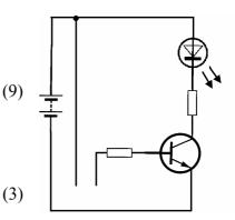
If the modified circuit was to be used to alert someone that a bath was full of water what component could replace the LED to make it more effective? (3)
