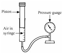
How could these measurements be used to find the *relationship* between pressure and volume for a gas?
